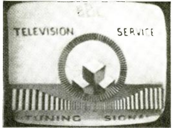
← Fig. 1. The distortion of the top part of this image is due to incorrect image-line synchronizing pulse application networks.
