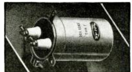
This type XAT-2 condenser is 1 of 3 television types in Solar's new line of oil-impregnated, oil-filled units, for use on circuits up to 7,500 V., D.C. Both leads are brought to terminals to permit grounding the can.
